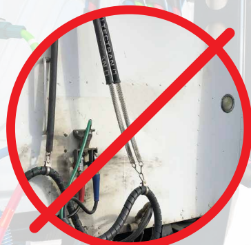
Springs should not be OVER stretched at rest
